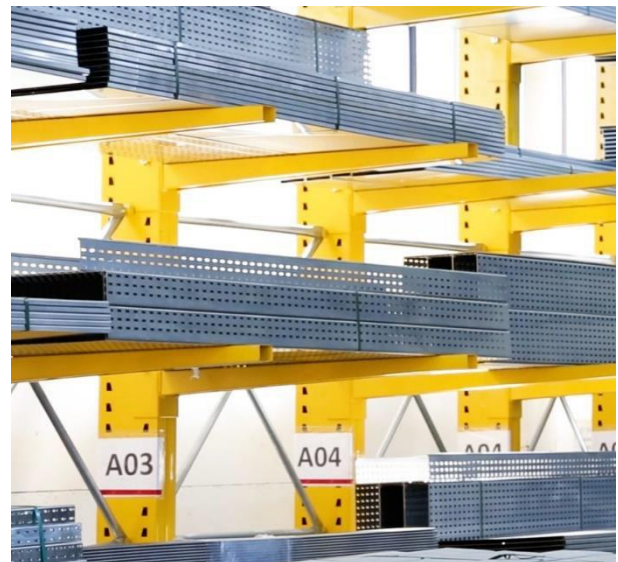
img.14c cable trays stacking
